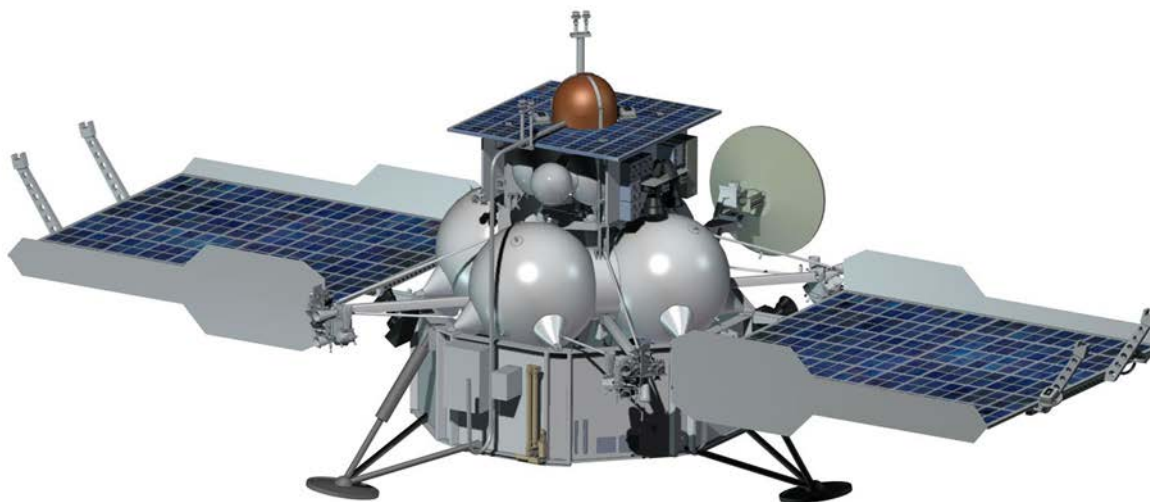
A simplified illustration of the Russian Fobos-Grunt lander package. The half-spherical object at the top was the descent capsule that would carry samples from the Martian moon Phobos back to Earth. Credit: ESA/Lavochkin Association
