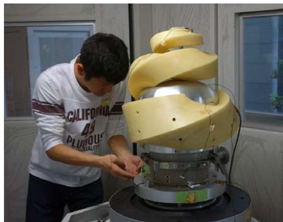
A full-scale prototype (engineering model) of DESPATCH. Credit: ArtSat
