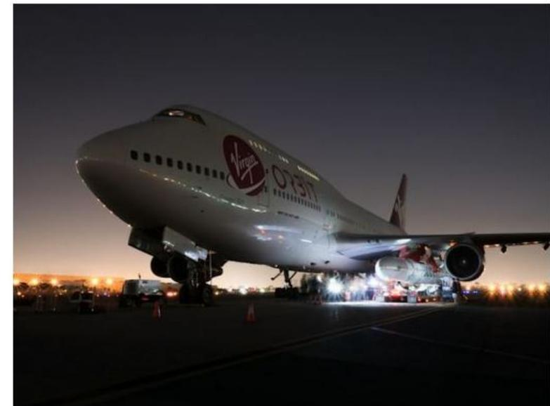
Launcher One attached to Cosmic Girl. The rocket attaches to a custom launch pylon underneath the portside wing. Image: Virgin Orbit.
